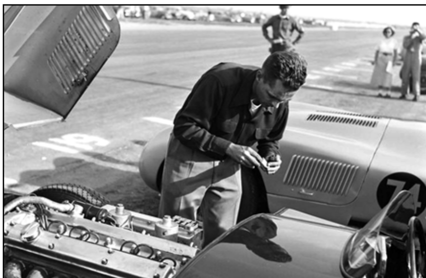
World Champion Phil Hill changes spark plugs on XJC 007 before the very first victory of a C-Type in America. He died on the 28th of August 2008.
