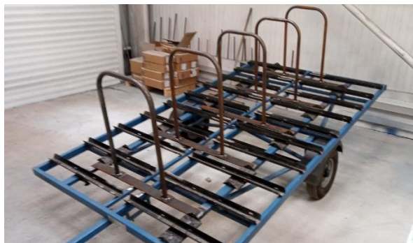
The Trailer during the recent refurbishment with hoops to secure the bikes.
